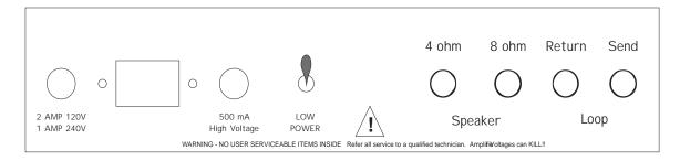
The Low Power switch, the speaker jacks and the jacks for the Passive effect loop switch are on the back panel.
